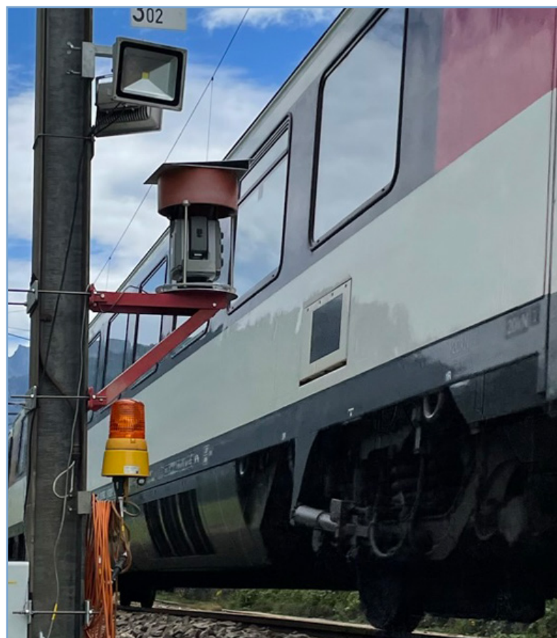
Monitoring of the left track over a length of 450m with five total stations
