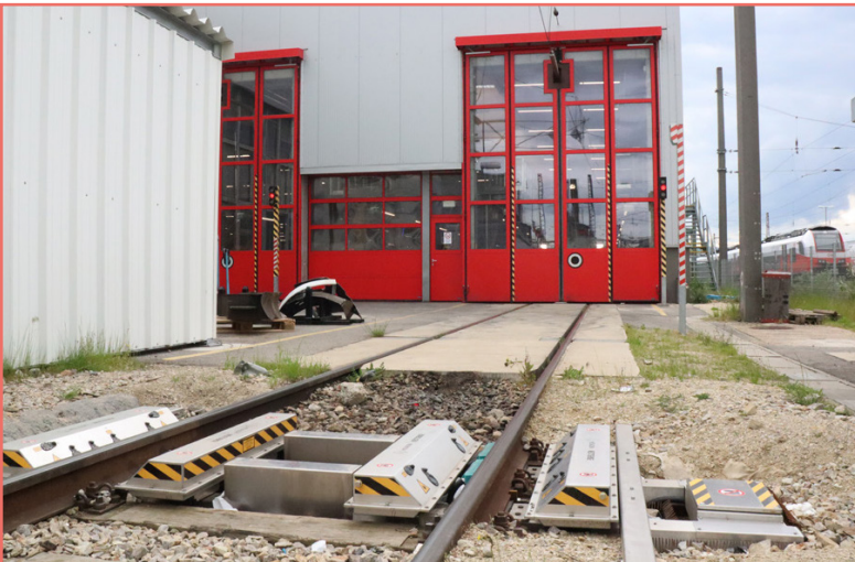
By the time the vehicle comes to a standstill in the hall, all wheelset data is already automatically saved in the system
