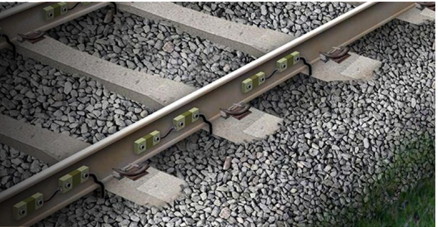
The accuracy of this system is based on measuring a complete train, consisting of a locomotive and various cars. Our AWIM system is equipped with eight weighing points. Formal tests by the Technical Research Institute of Sweden show even an average accuracy of  $\pm 0,2\%$ . When combining all measurements an overall accuracy of better than  $\pm 0,5\%$  is achieved for passing trains with various speeds, complying with OIML R106, class 0,5.
