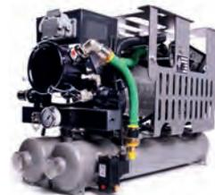
This system is designed for lubricating the wheel flanges of streetcars. The system works on the principle of applying a lubricant mixture to the contact area between the wheel flanges and the rails by means of pressurized air.
