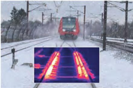
In climatic regions which frequently experience temperatures below freezing, malfunctions of railroad rail switch mechanisms is often a problem. Temperatures below freezing and the accumulation of snow and ice result in issues with railroad switch mechanisms.
