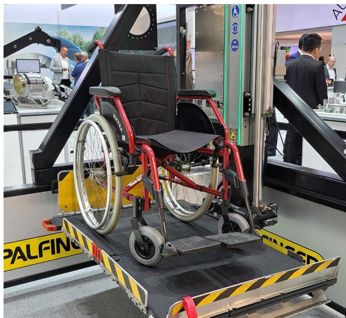
been designed with high-speed and commuter trains in mind. A key advantage of this swivel lift is its ability to be fully stored and hidden behind cover elements.
