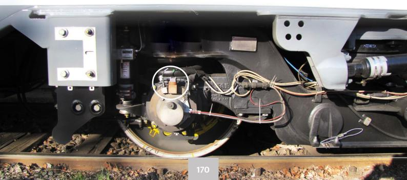
Pre-qualified accelerometers of type ASC RAIL-x152LN
