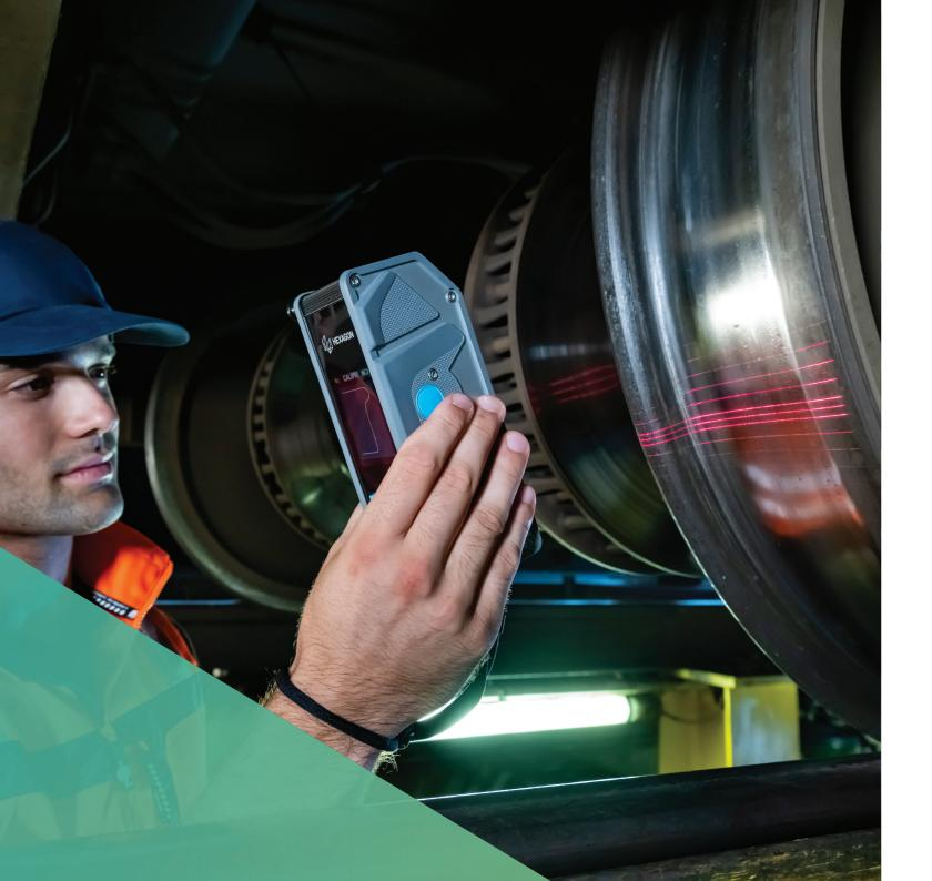
Handheld optical inspection solution for railway wheel profile dimensions
