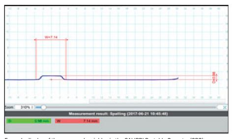
Example display of the measured variables in the CALIPRI Portable Operator (CPO)
