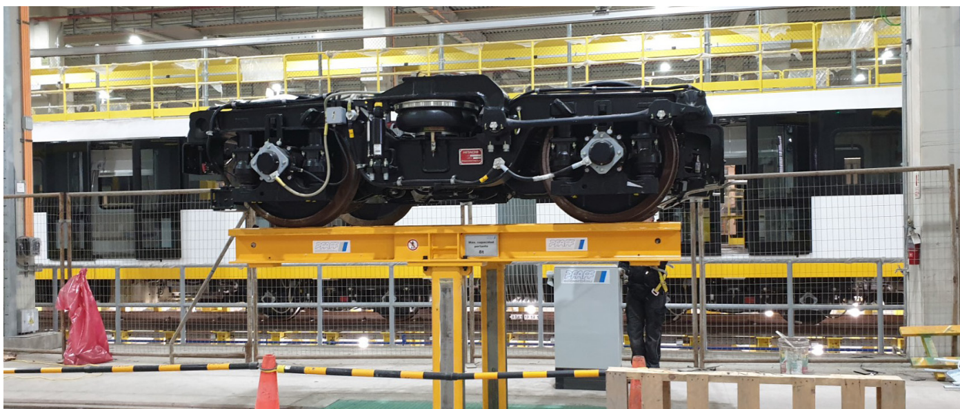
Underfloor bogie lifting stands in Peru
