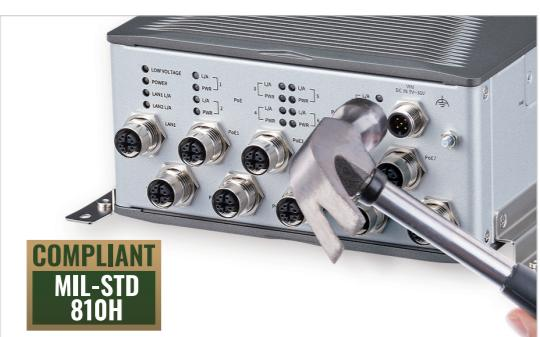
Ultra-rugged enclosure, comply with MIL-STD-810H against vibration and shock impact
