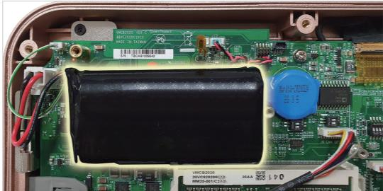
Back-up battery provides uninterrupted power
