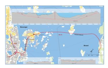
tunnel, spanning 14.3 kilometres and reaching 291 metres below sea level at its deepest point.
