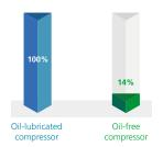
Total maintenance costs per compressor over a period of 20 years based on a real project comparison.
