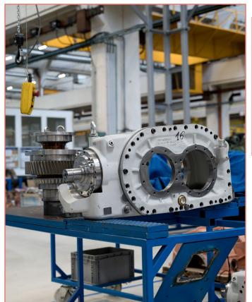
helical gearboxes with a solid or hollow shaft are mostly used, it can be said that the Wikov MGI + Gmeinder Getriebe duo covers, with exceptions, all bogie concepts used in modern trams.
