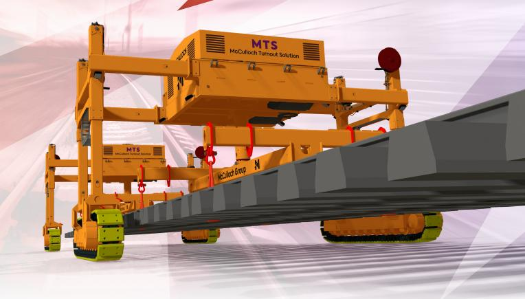
**The MTS can access and egress almost anywhere on track.** It can move with ease pre-built panels in any direction before installation, allowing you to handle S&C installation with ease. The MTS also removes the need for large work areas, or temporary track along with associated planning challenges.
