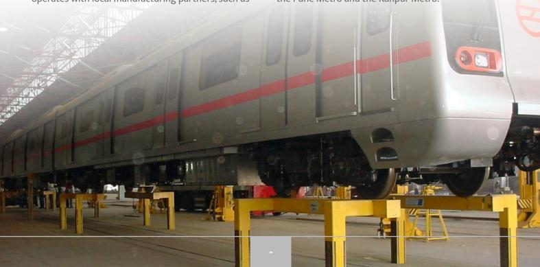
The pre-assembled system, which was accepted in Ahmedabad, is currently on its way to HYT Engineering, where it will be prepared for final assembly at the Shakurbasti depot near New Delhi. From the end of 2023, it will be used there for the maintenance and servicing of eight-carriage Vande Bharat trains. The end user of the lifting system is the state-owned railway company Indian Railways. It operates most of the nationwide rail transport.
