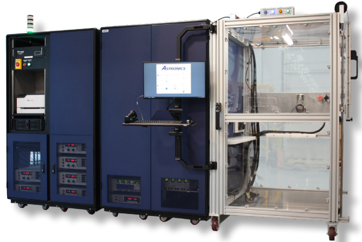
ATS-500 High Power Test System
