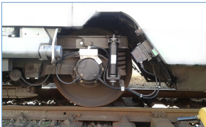
Installed DB Systemtechnik sensorbox mounted on the wheelset
