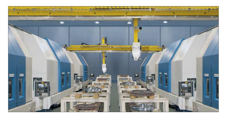
The Niles-Simmons RQ-Series Vertical Turning Centers with one or two ram heads were conceived for heavy duty cutting of railway wheels. Robust design, use of heavyduty cutting tools with Capto C10 interface, and automatic tool change ensure optimum machining of forged or hot-rolled railway wheels.
