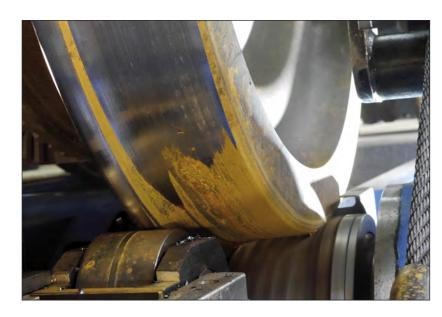
The **Stanray**<sup>®</sup> wheel truing product line has been an essential part of railway maintenance facilities since 1949. Freight and transit railways worldwide owe their wheel sets' safe and efficient operation to the Stanray's rugged reliability.
