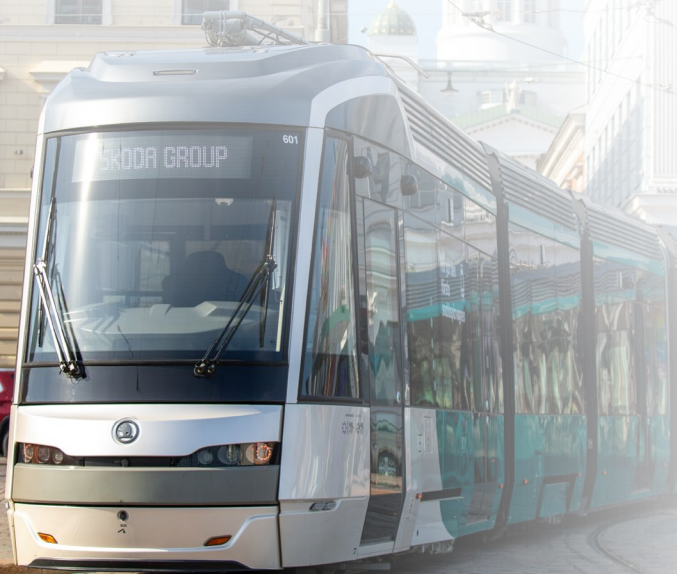
New multi-articulated tram with pivoting bogies Škoda Artic X54
