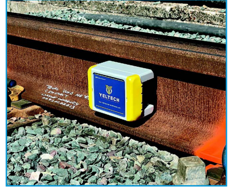
Rail Temperature Monitor
