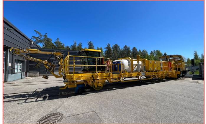
Tunnel-cleaning wagon manufactured by VR FleetCare
