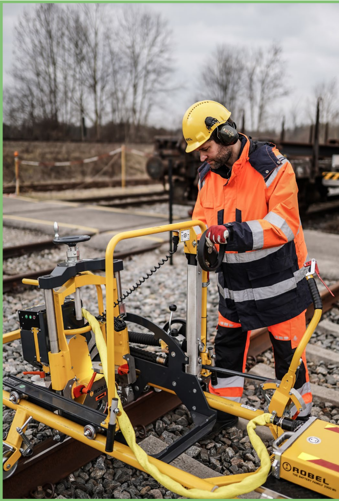
One frame, eight modules, covering all grinding applications on track © Robel
