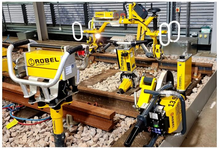
The battery-powered E<sup>3</sup> construction site – from left: ROTAMP 62.20L, ROGRIND 13.49, ROMPACT 30.20, ROCUT 13.90 © Robel
