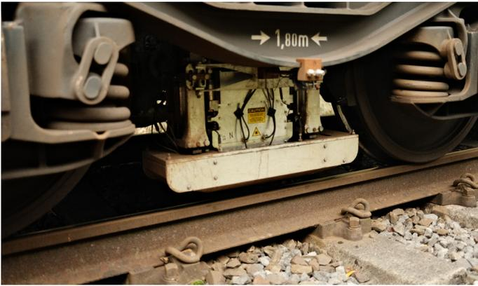
system to switch automatically between modes and avoid hitting rail obstacles.
