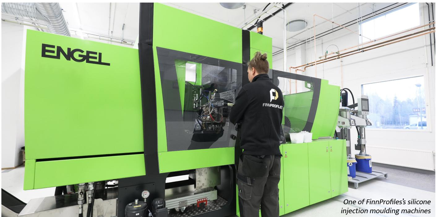
*One of FinnProfiles’s silicone injection moulding machines*
