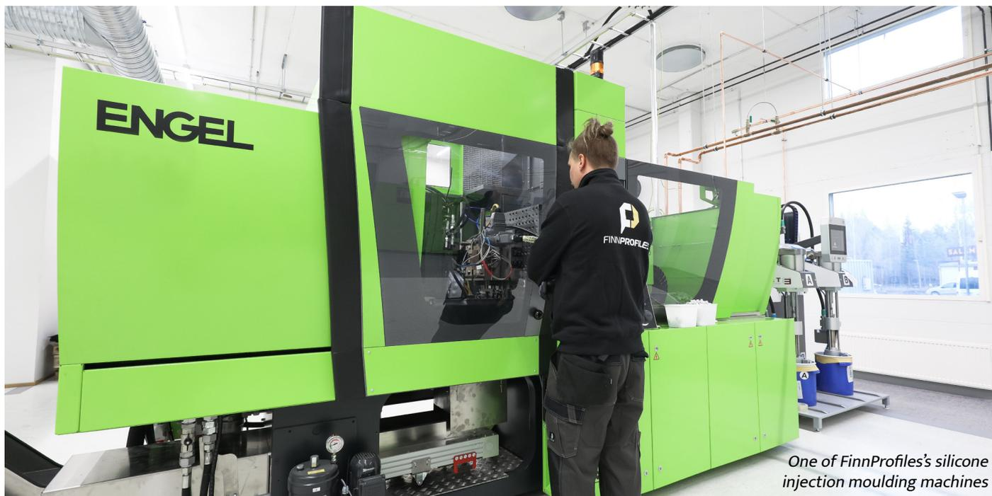
*One of FinnProfiles’s silicone injection moulding machines*
