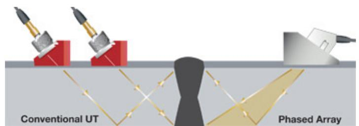
value than traditional UT because a single PAUT probe is able to test multiple angles and depths, scanning all critical areas during a one-rotation scan.
