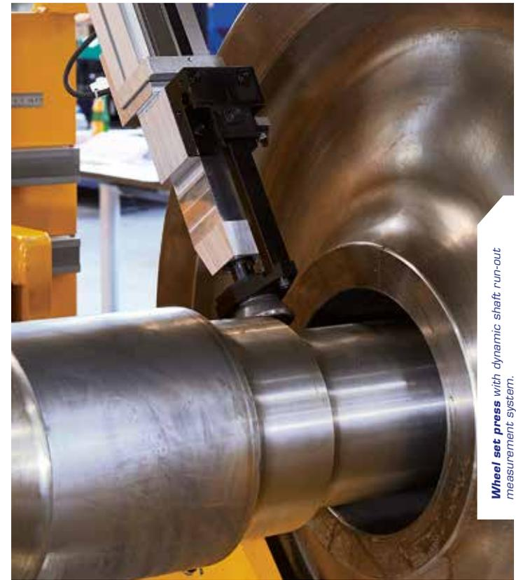
**Wheel set press** with dynamic shaft run-out measurement system.
