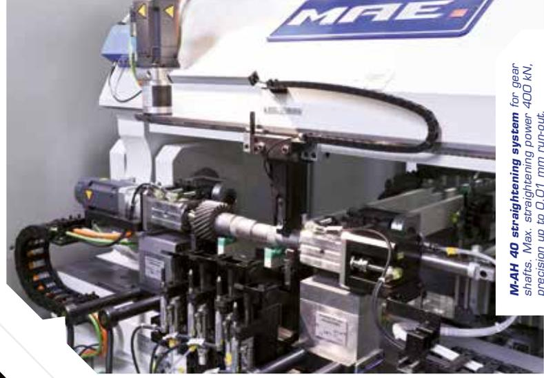
**M-AH 40 straightening system** for gear shafts. Max. straightening power 400 kN, precision up to 0,01 mm run-out.
