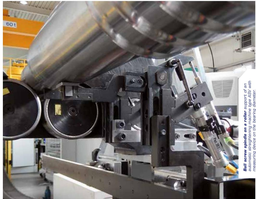
**Ball screw spindle on a roller** support of an
