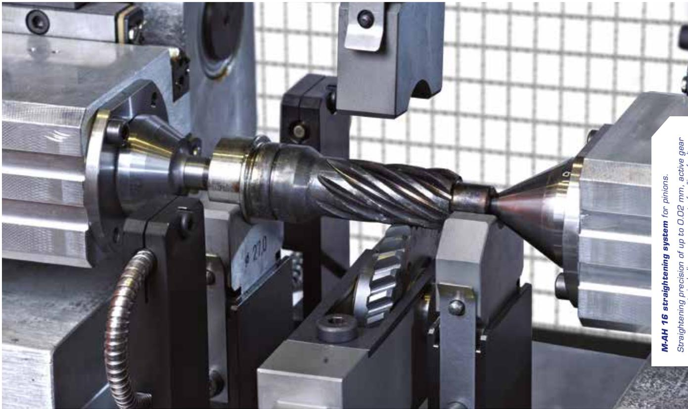
**M-AH 16 straightening system** for pinions.
