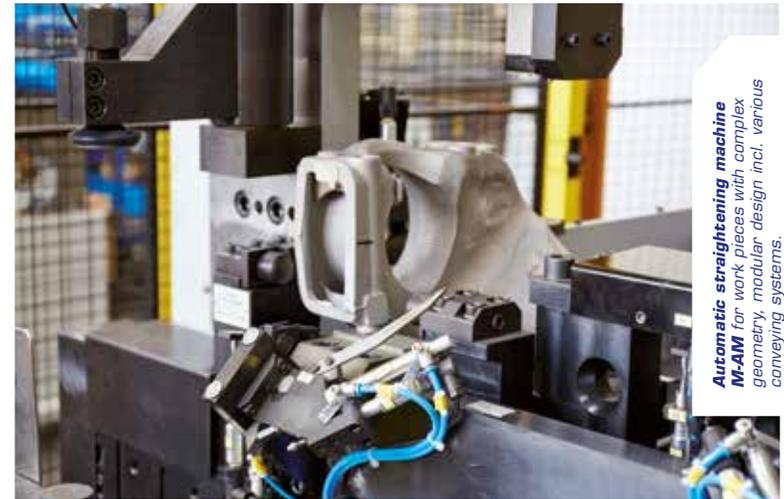
**Automatic straightening machine M-AM** for work pieces with complex geometry, modular design incl. various conveying systems.
