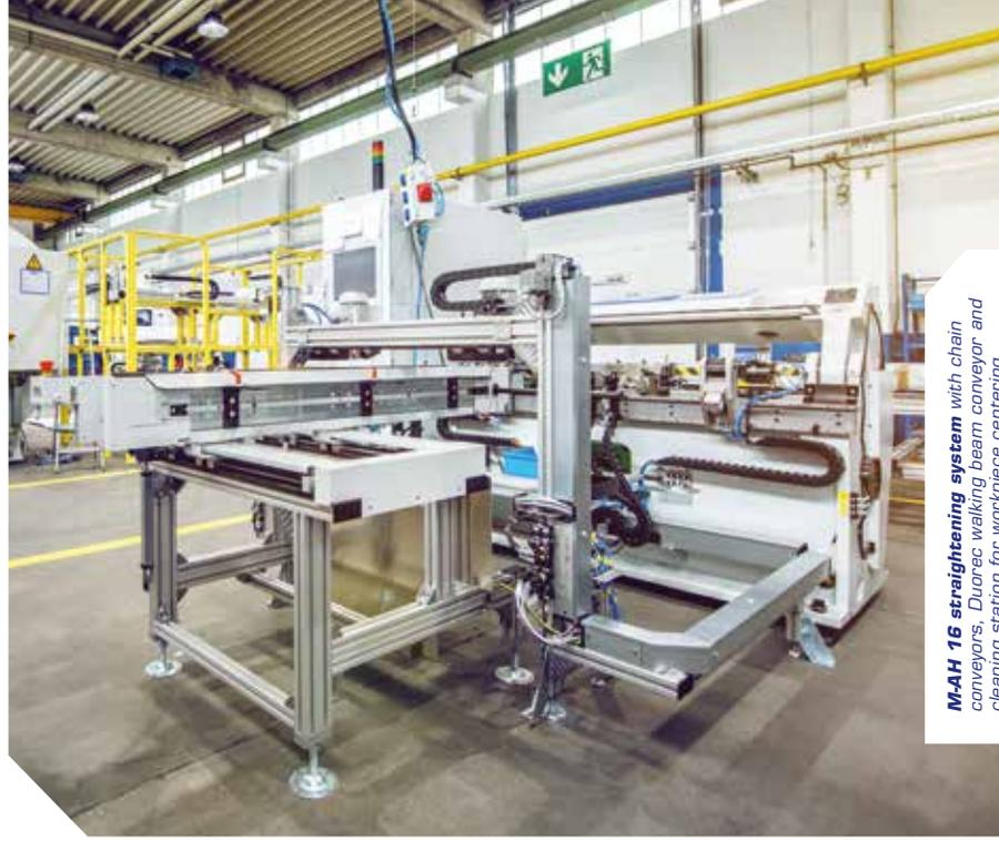
**M-AH 16 straightening system** with chain conveyors, Duorec walking beam conveyor and cleaning station for workpiece centering.
