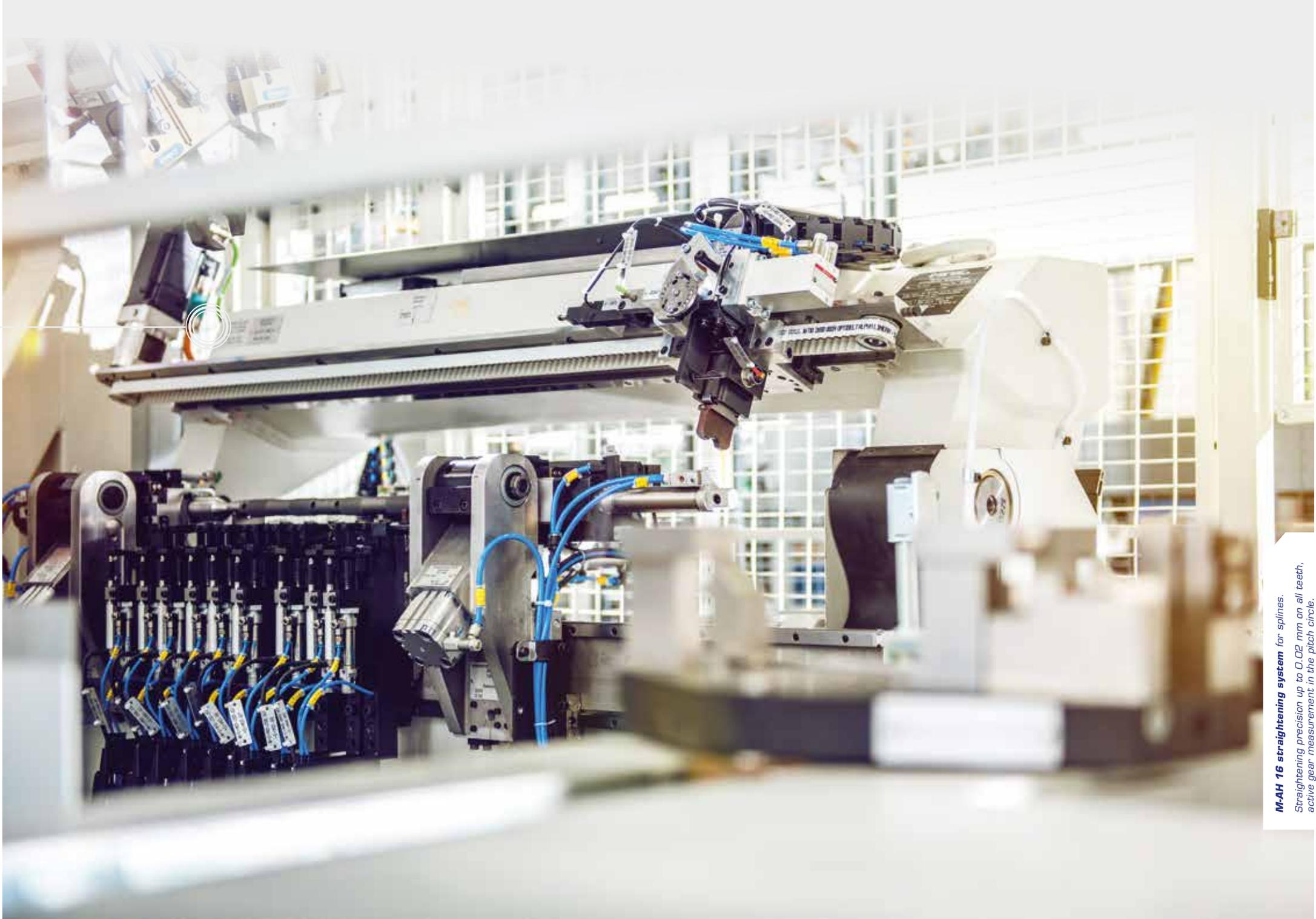
**MAH 16 straightening system** for splines.
