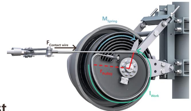
$$F_{\text{Contact wire}} = \left( f \frac{M}{r} \right) = \text{const.}$$
