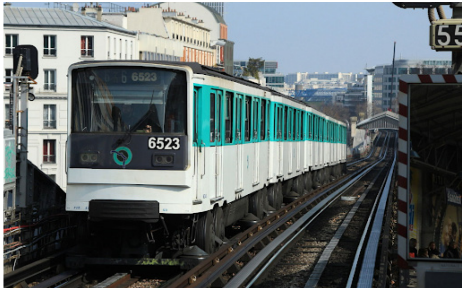
Train on tyres (MP 73) of Line 6 of the Paris metro
