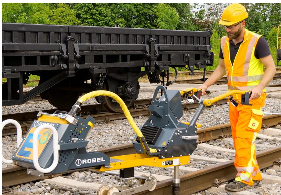
Fully electric precision power wrench ROWRENCH 30.76 E<sup>3</sup>
