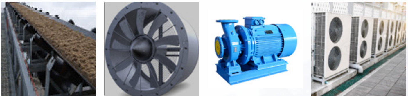
Fig 1.- Typical applications of three phase induction motors
