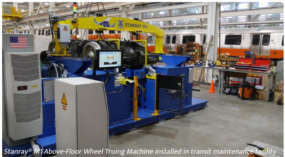
Stanray® M1 Above-Floor Wheel Truing Machine installed in transit maintenance facility
