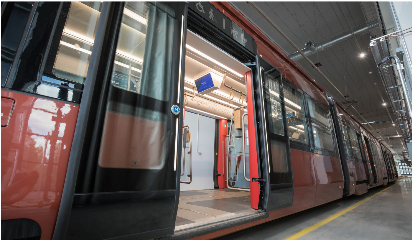
Tampere's trams in Finland include 320 door seals, all made by FinnProfiles. In addition, all doorstep rubbers are made by the company. The material that has been used in these products is a fire-safe EPDM rubber, approved according to the EN45545-2 standard.
