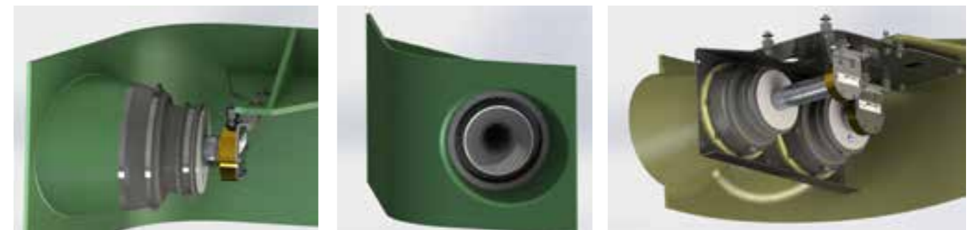
Fig. 03/04 The sound insulation is pushed in, for example, via a connecting socket on the side of the vehicle. In this way, the Makrofon is kept facing forwards and is additionally fitted to the Makrofon cover using rubber-metal mounts. The sound insulation reduces the sound pressure level in the driver's cabin by ensuring that the sound only propagates forwards.
