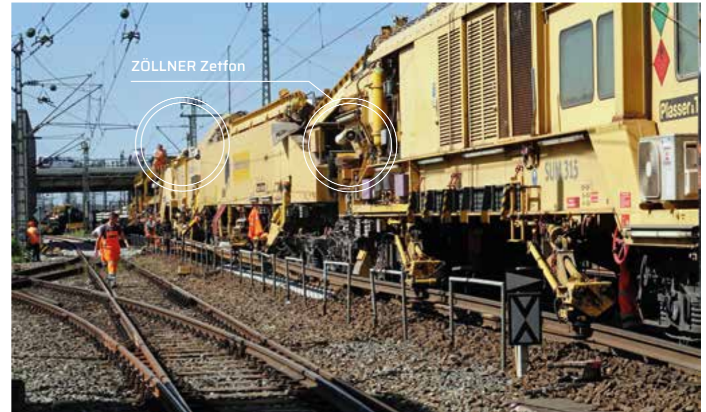
Fig. Example of a ZET FON on a high-output track renewal train
