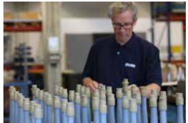
Fig. A look inside our workshop: assembly of Makrofonen of the ZM75 series. Only perfectly manufactured signal horns receive the ZÖLLNER inspection stamp.
