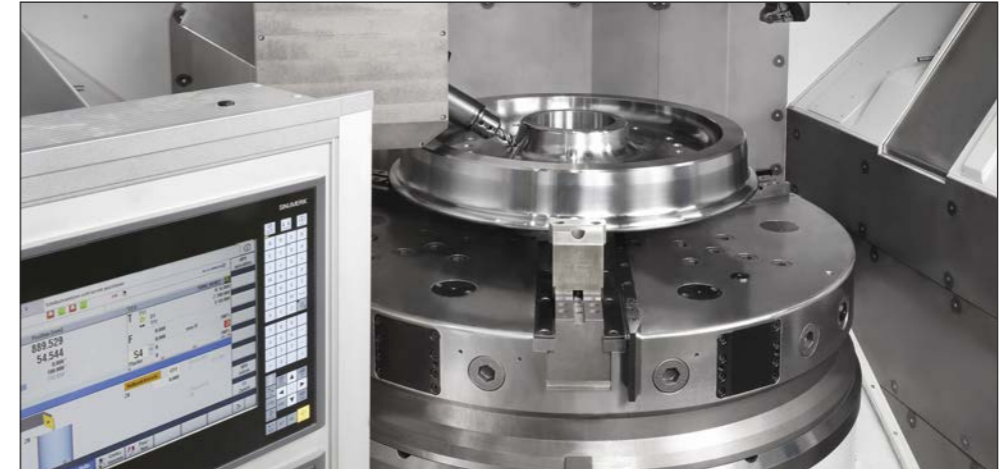
The Niles-Simmons RQ-Series Vertical Turning Centers with one or two ram heads were conceived for heavy duty cutting of railway wheels. Robust design, use of heavy-duty cutting tools with Capto C10 interface, and automatic tool change ensure optimum machining of forged or hot-rolled railway wheels.
