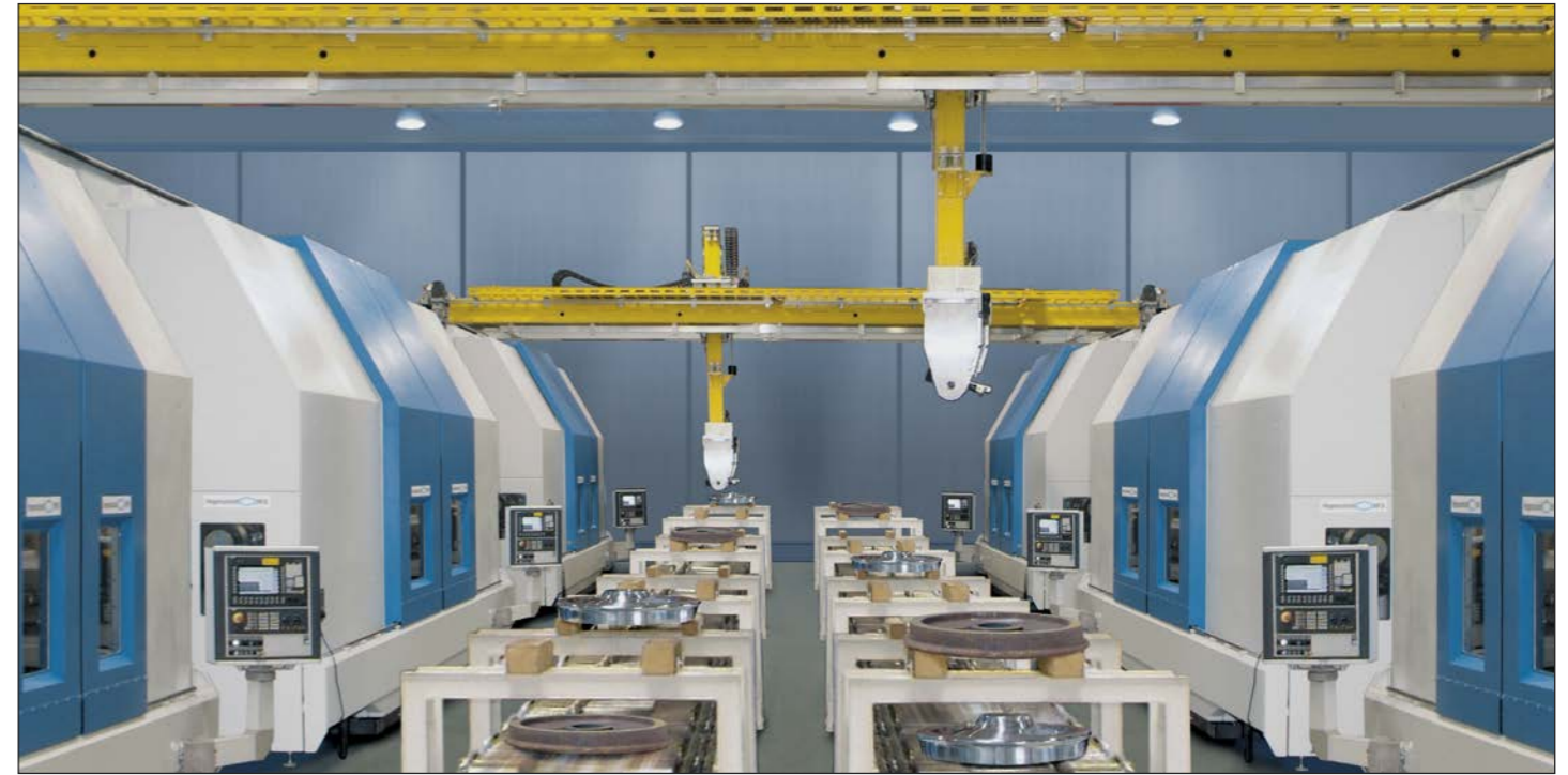
The Niles-Simmons RQ-Series Vertical Turning Centers with one or two ram heads were conceived for heavy duty cutting of railway wheels. Robust design, use of heavy-duty cutting tools with Capto C10 interface, and automatic tool change ensure optimum machining of forged or hot-rolled railway wheels.
