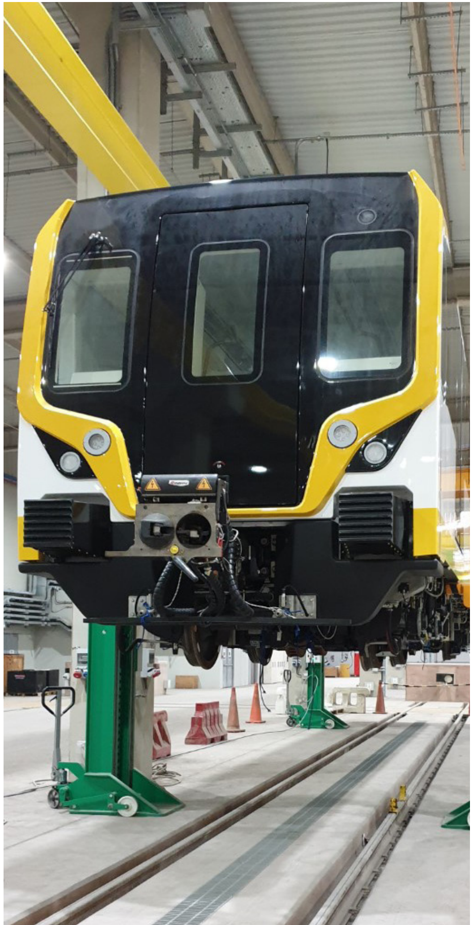
Pfaff Verkehrstechnik has successfully completed a major contract for the new Metro Lima depot in Peru, which includes mobile lifting jacks for lifting individual uncoupled carriages
