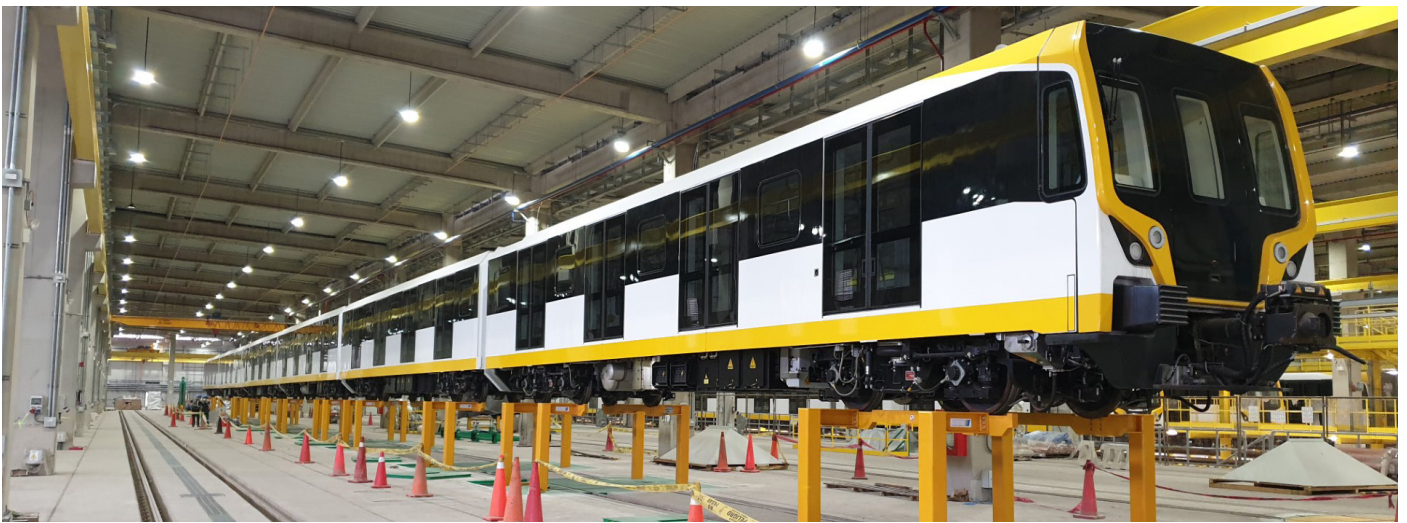
Underfloor lifting system for heavy trains with up to seven carriages and a length of 120m
