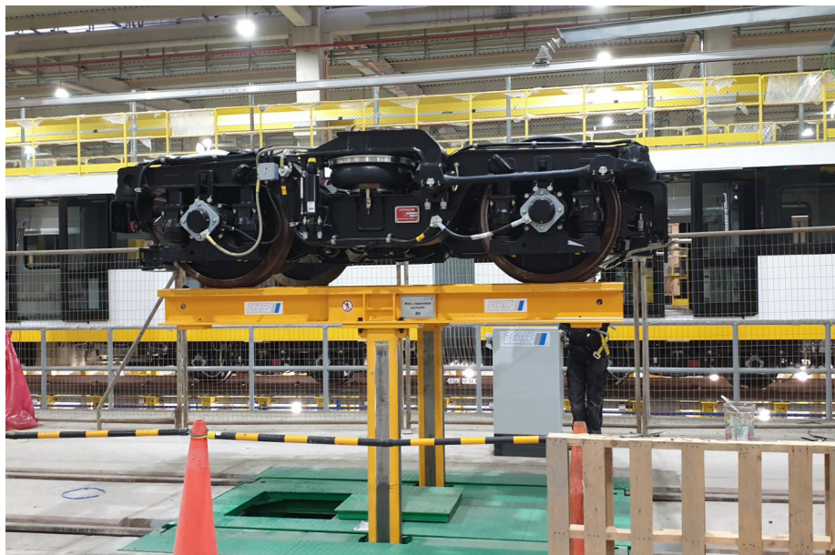
Maintenance and repair work on the bogies is carried out with underfloor bogie lifting stands
