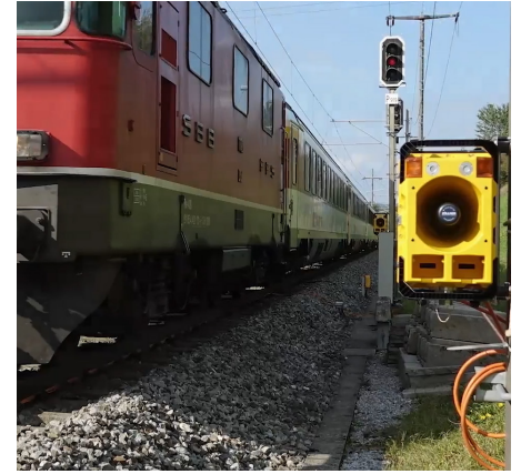
Image 3 ZPW126-31 mounted using magnet fastening
