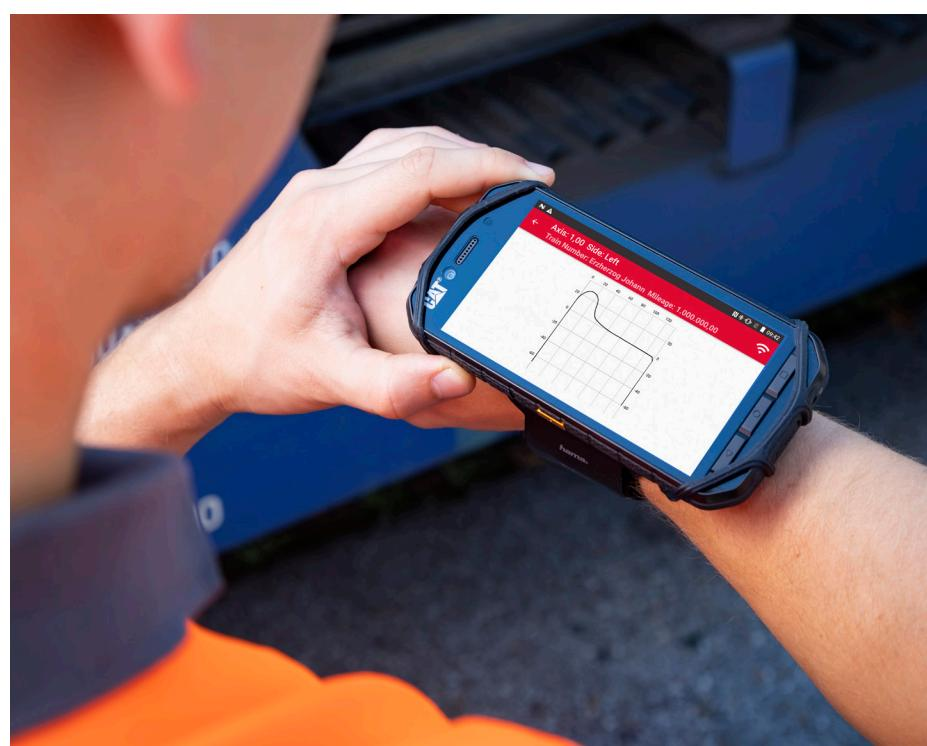
Figure 5: View of the wheel profile as point curve
