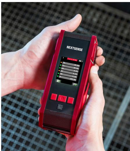
Figure 3: Colour-coded measured variables on the sensor
