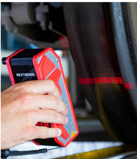
Figure 2: Contact-free measurement of the wheel profile
