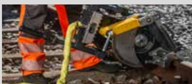
ROCUT 13.90 E 3 Electrical Rail Cutter
