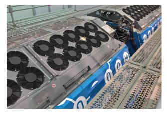
Multiple core fuel cell stacks are combined, sharing integrated cooling, ventilation and output regulation.
