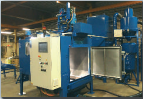
A blasting cabinet with a robotic blasting device. Blasting media is ceramic beads and dry ice.
