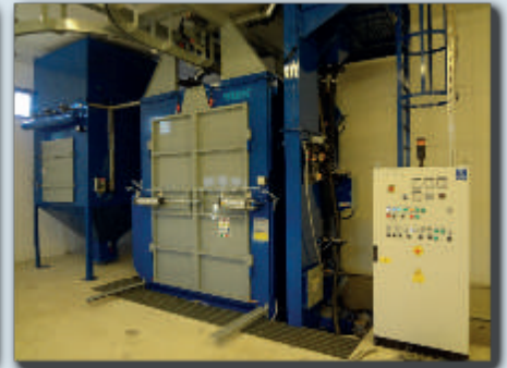
An overhead conveyor wheel blast machine with 3 blast wheels.
