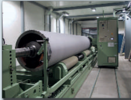
A blasting room with a fully automated blasting device for large rolls.
