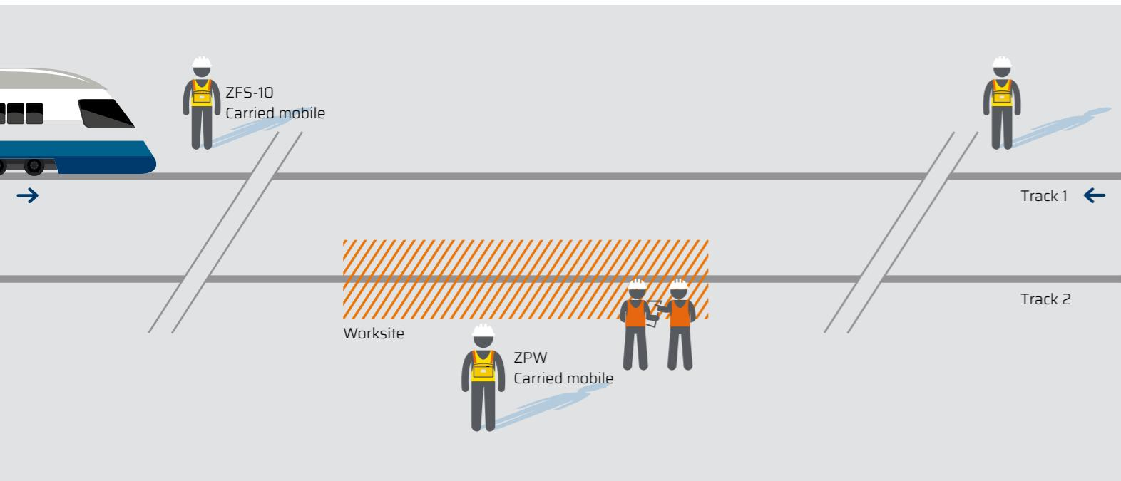
**Fig. above** The double function of the ZPW as a warning device and a control unit reduces material expenditure to a minimum.
