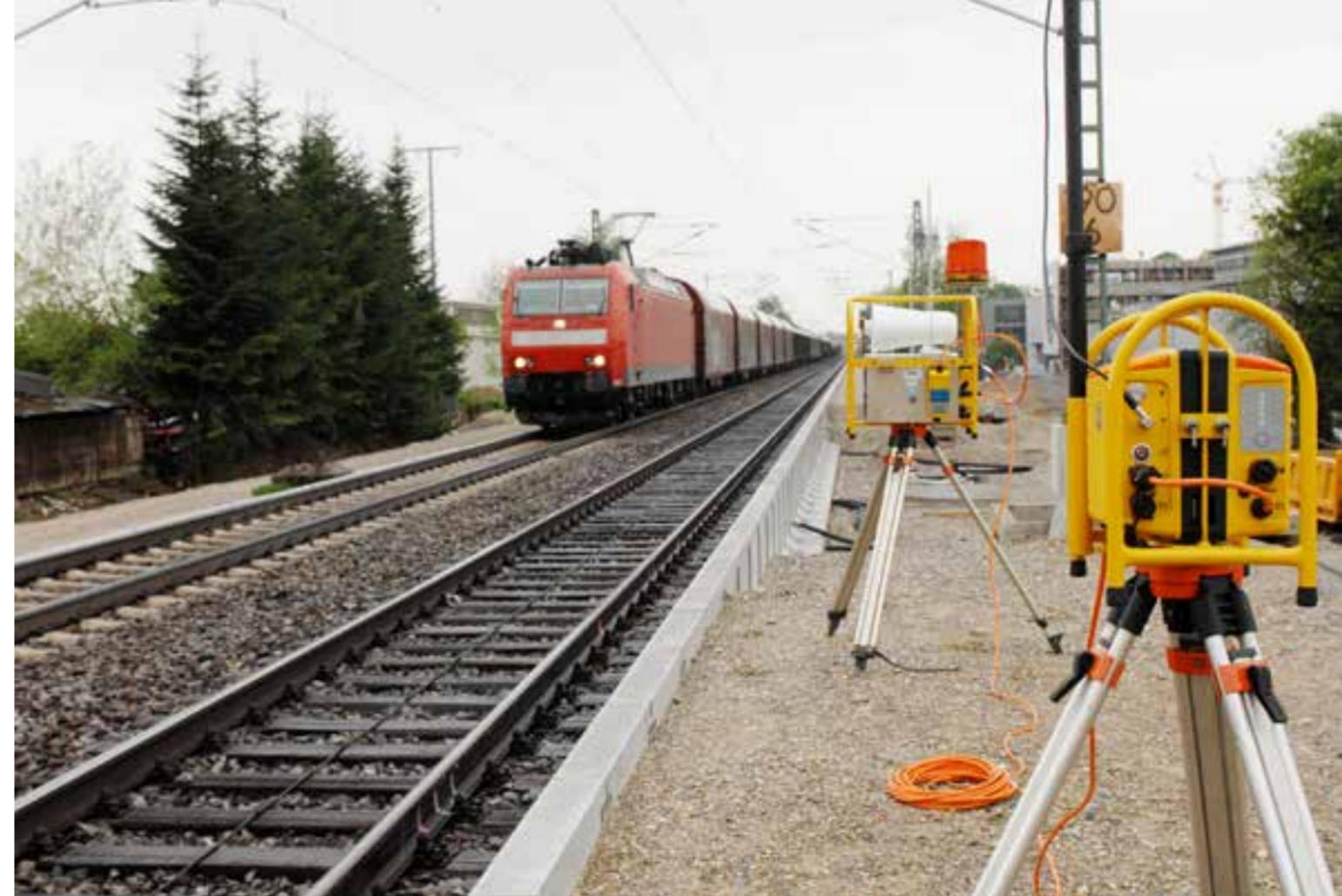
Fig. above The WGH/WGL warning device is integrated into the MRWS via connection to the ZPW.
