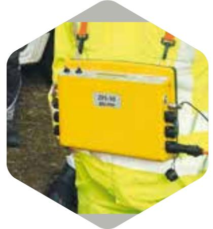
Trains in motion are detected either using rail contacts embedded in the track or manually by a safety monitor. In both cases, the radio transmitter ZFS transmits the information on the upcoming train in motion to the worksite, where the warning signal issue is triggered. After the railway vehicle has passed the worksite, the warning is cancelled, and work can continue.
