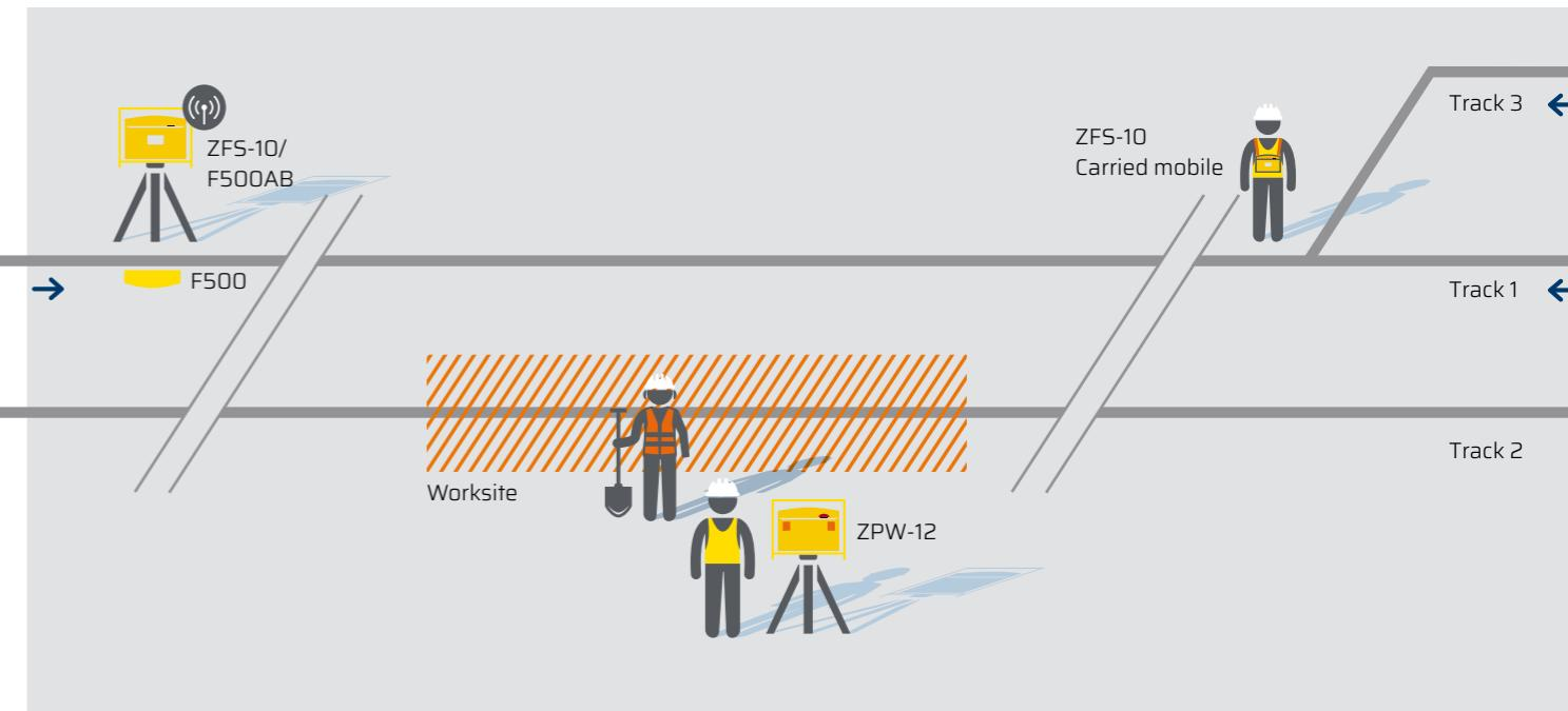
**Fig. above** Depending on the situation at the activation point, the warning can be triggered either manually using the ZFS or automatically using a train detector.
