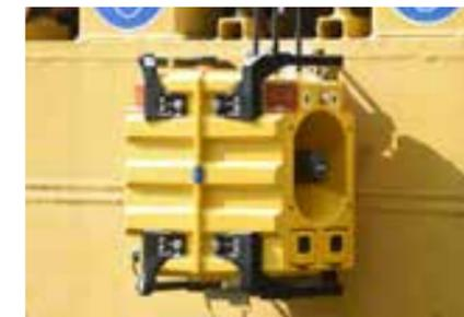
**Fig.** The ZPW126-10 can also be used as a mobile warning device on track construction machines or can actuate the machine's own warning system using the integrated ERRI interface.
