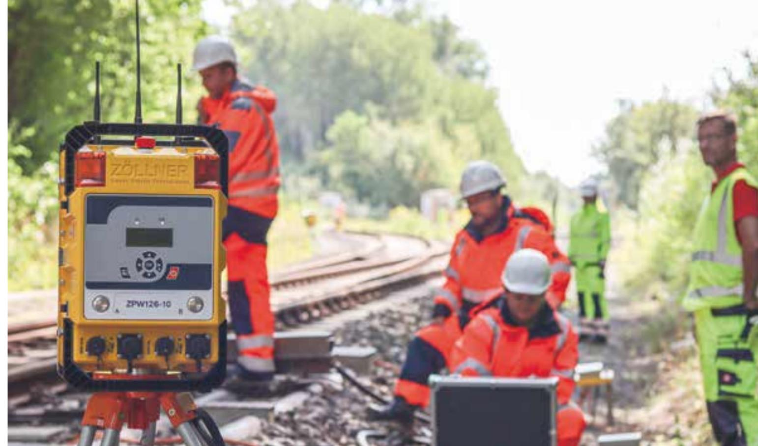
LEDs on every corner of the housing guarantee 360°, all-around perceptibility, and the ready indicators provide information on the operational readiness of the system at all times. The ZPW126-10 can function either as a master or remote. Actuation of the ZPW126-10 in master operation makes it possible to incorporate an unlimited number of warning device groups, each with up to five remote warning devices (see the graphic on the following page).
