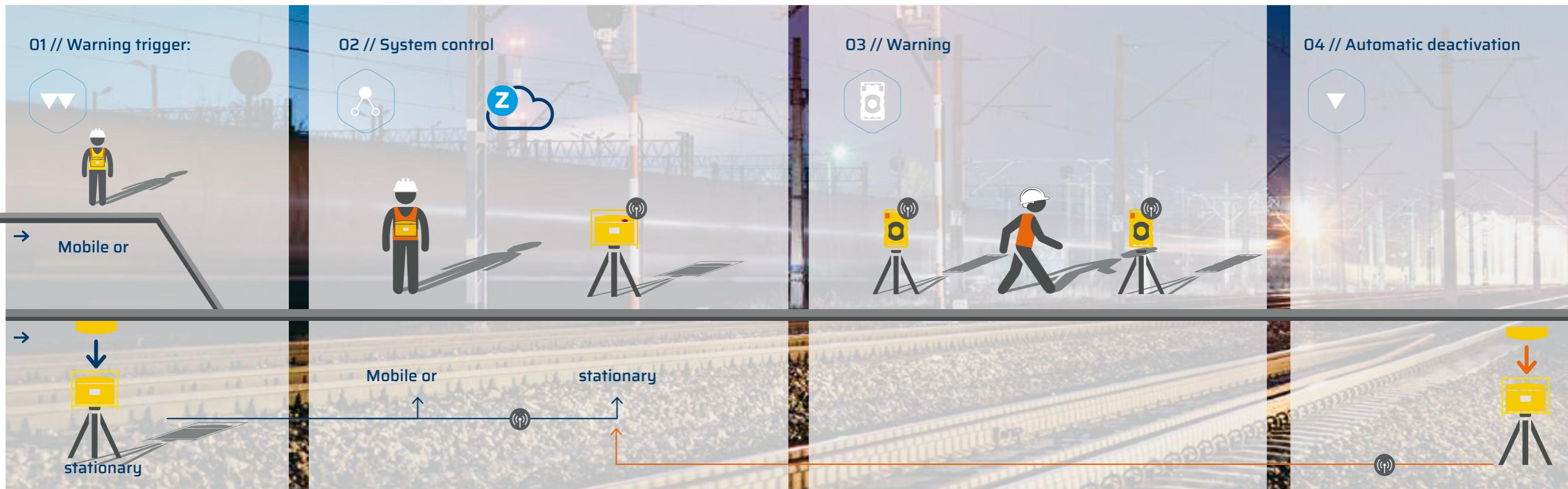
The warning can be triggered automatically, and/or it can be triggered manually via a mobile radio transmitter.
