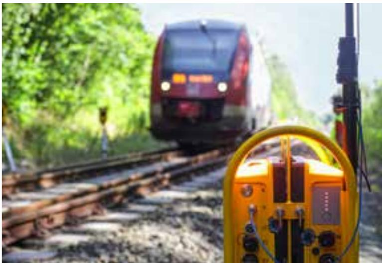
**Figures above** The ZPW can be both carried mobile and used as a stationary unit on a stand.
