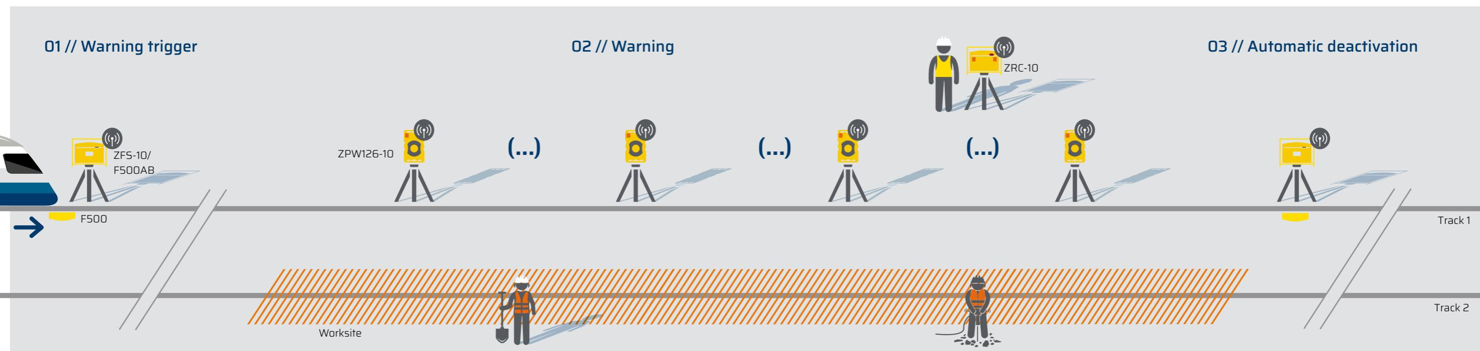
**Fig. below** Longer worksites can also be optimally protected with the ZPW126-10.
