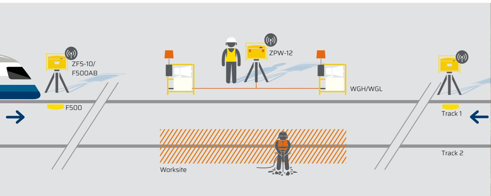
**Fig. above** For especially loud work, two WGH/WGL can be connected to each ZPW to warn all employees with a warning signal of up to 126 dB(A) that is sure to be heard.
