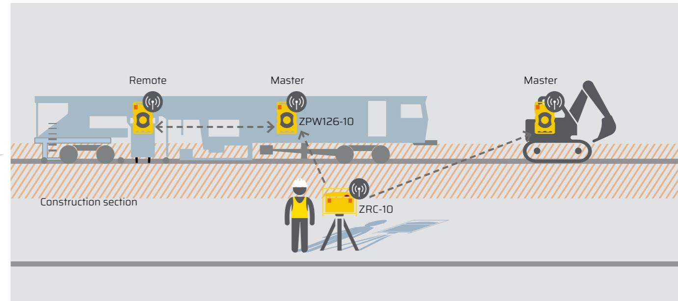
**Fig. above** The ZPW126-10 can be attached directly to a machine or an excavator using the magnetic holder and function as part of a warning device group and/or, as an alternative, actuate the machine's own warning system via its ERRI interface. The ZPW126-10 master and remote on the machine form a warning device group. On the excavator, the ZPW126-10 constitutes its own warning device group.
