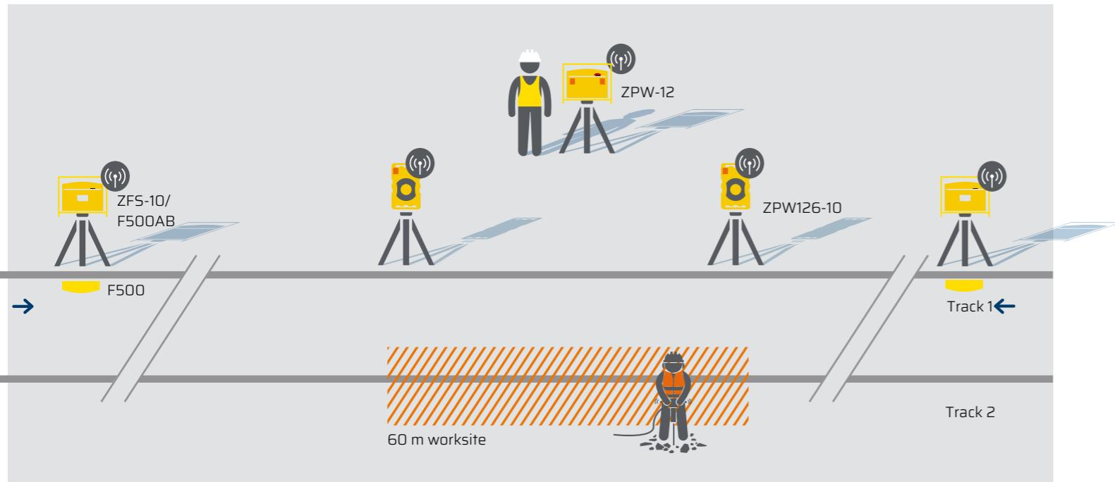
**Fig. above** For smaller or loud worksites, the ZPW126-10 is used at certain points as a warning device. The warning can be triggered automatically - as depicted - manually or a combination of both.
