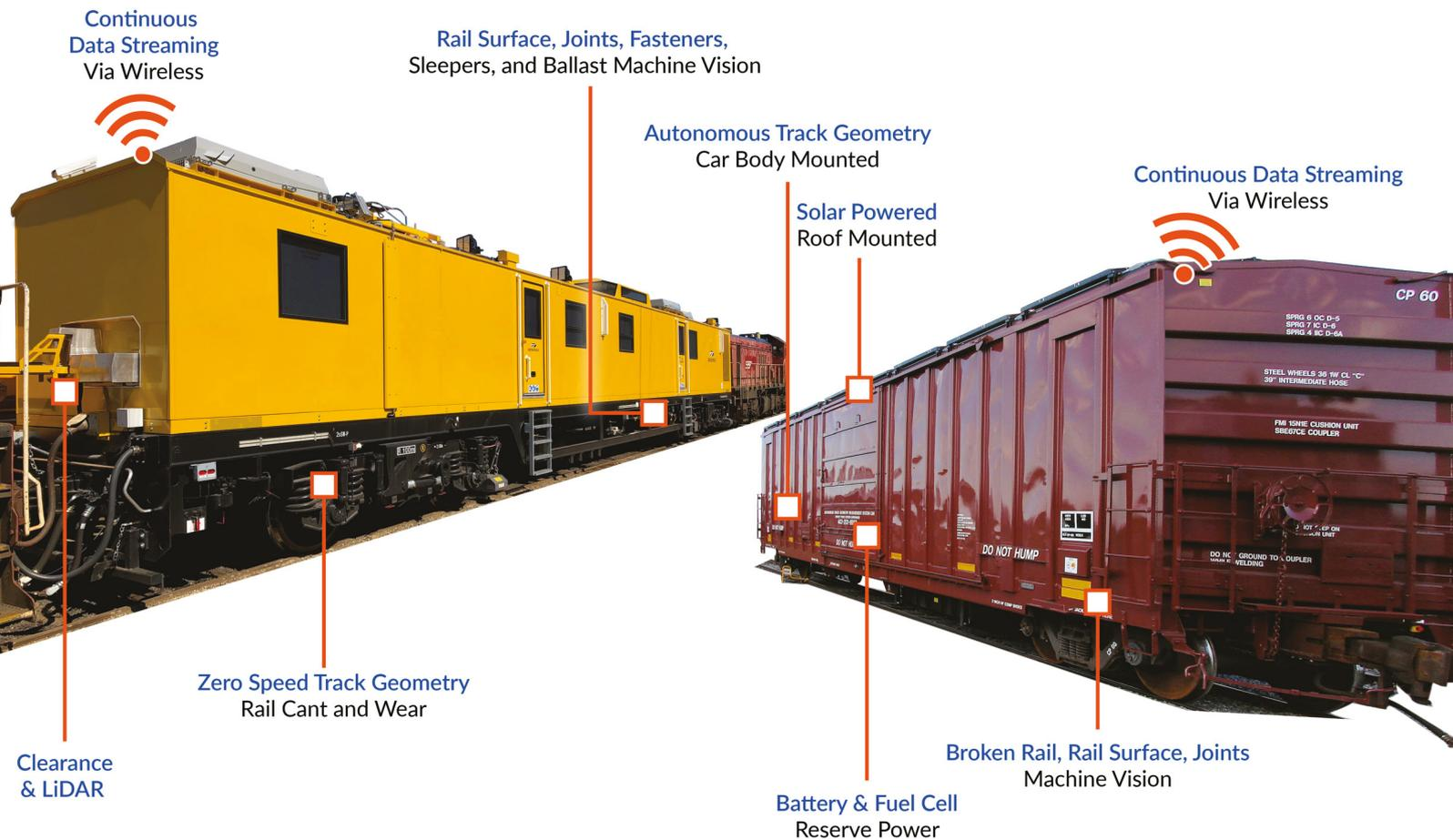
ENSCO Rail is the premier provider of autonomous inspection systems that identify defects early and improve rail network safety – at the lowest cost per inspection.
