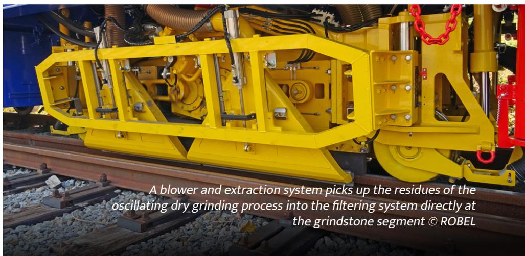
*A blower and extraction system picks up the residues of the oscillating dry grinding process into the filtering system directly at the grindstone segment © ROBEL*
