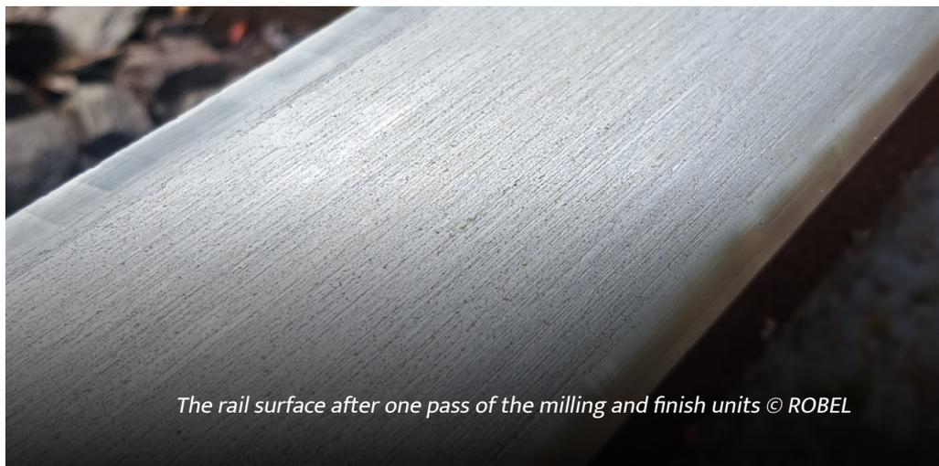
*The rail surface after one pass of the milling and finish units © ROBEL*
