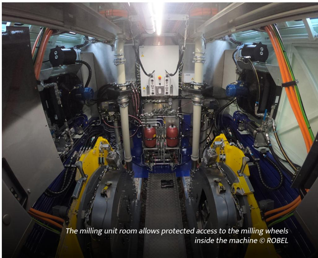
*The milling unit room allows protected access to the milling wheels inside the machine © ROBEL*
