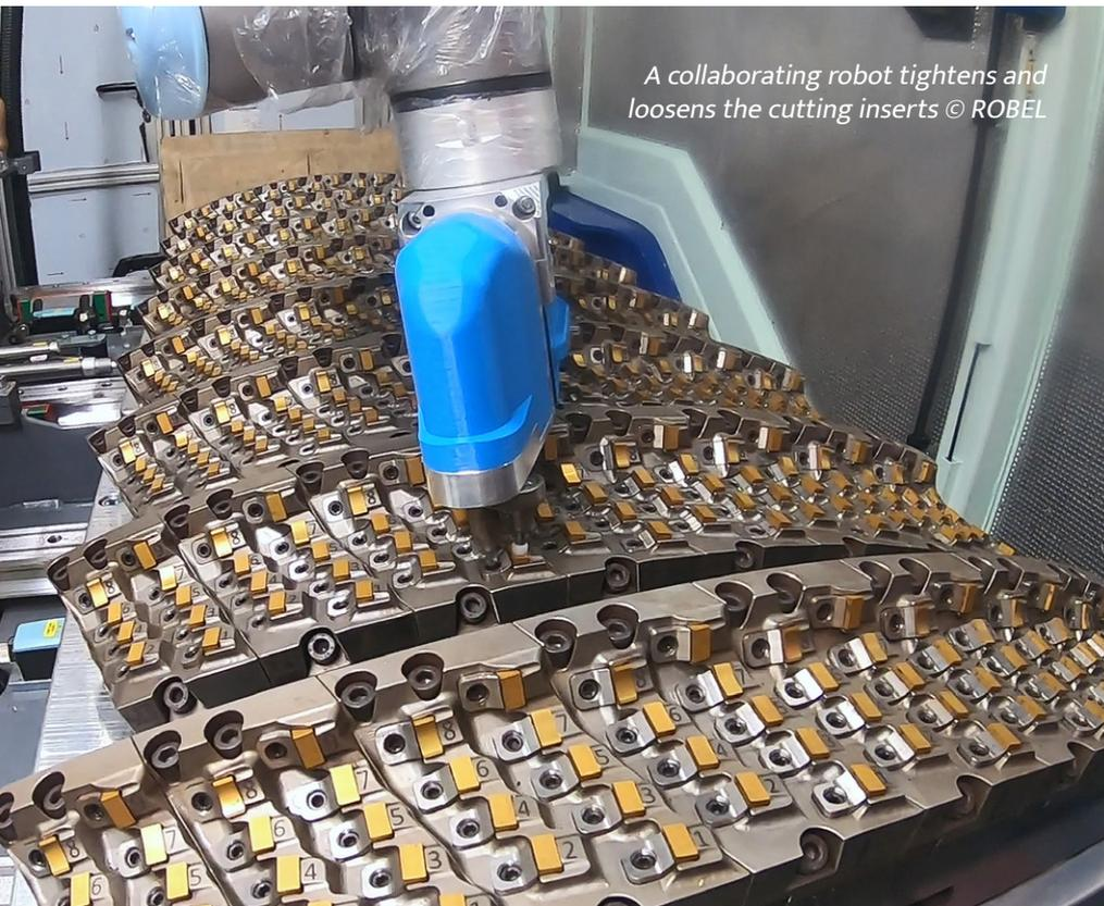
*A collaborating robot tightens and loosens the cutting inserts © ROBEL*
