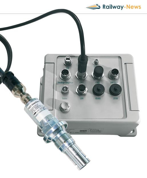
but also to prevent it, if possible. The overwhelming majority of all damage to gearboxes is caused by missing or incorrect lubrication, which can be avoided by continuous monitoring and timely replacement of the oil. As a multi-criteria sensor, the GGT GearSaver<sup>®</sup> monitors a large number of relevant physical quantities that provide information about the condition of the gear oil.
