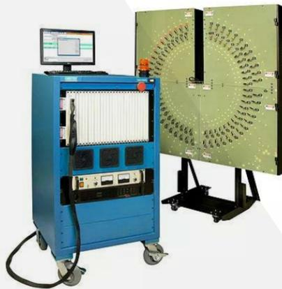
Bulk Wire Analyzers use a proprietary high voltage switching architecture to evaluate and test reels of bundled twisted-pair cable up to 30,000 feet in length for conductor resistance, insulation resistance, conductor to conductor dielectric strength up to 10 kVDC and core to sheath dielectric strength up to 15 kVDC. AC High Voltage testing is available (as a standard offering) up to 6000VAC for 30,000 foot cables.
