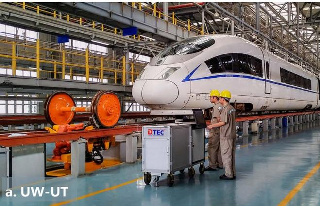
Our Underfloor Wheelset Ultrasonic Testing System (UW-UT) is designed to perform highly efficient, accurate, and highly reliable wheelset inspections under the train. With our Underfloor Vehicle Bogie Machine Vision System (UVB-MV) using Artificial Intelligence, 3D imaging, and robotic automation techniques, we are moving the asset management into a new era of smart maintenance.
