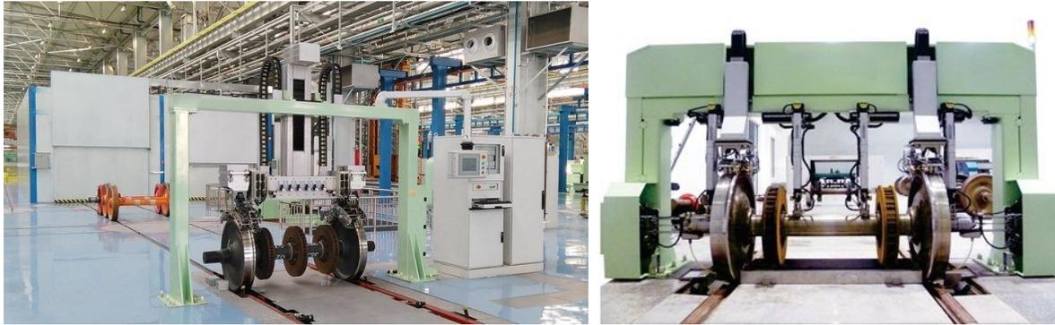
*Dismounted wheelset and solid axle ultrasonic testing systems*
