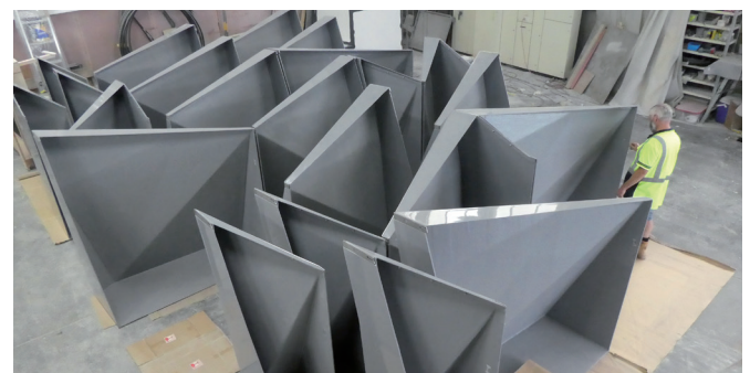
Top: The interlocking screens in situ Bottom: Completed screens awaiting installation
