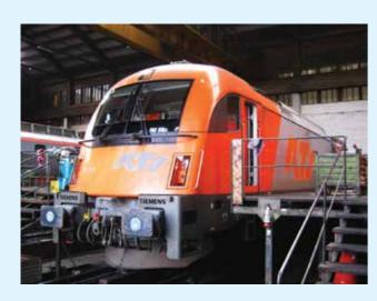
One of their locomotives, a Siemens Taurus (ES 64 U4) electric locomotive labelled Class 1216-901, arrived to Center Ljubljana for a P12 control check all the way from Croatia, where it runs service on a track-renewal construction site. As this particular model is almost identical to SŽ Class 541, the work on the orange newcomer largely followed the usual practice applied to SŽ locomotives of this type.
