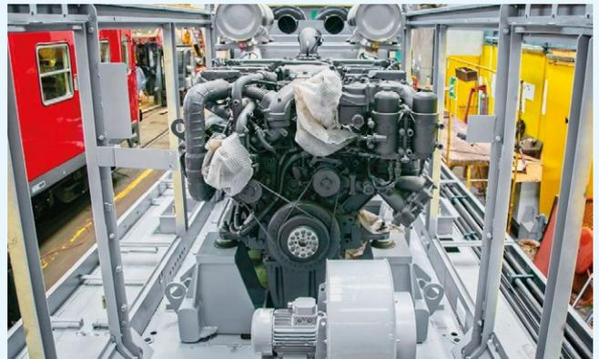
At SŽ – VIT, we have been working to modernize Slovenske železnice's rolling stock for a number of years now, which included, amongst other, upgrading and repowering Class 642 and 643 locomotives. In an effort to increase vehicle availability, cut maintenance costs and lower emissions, the locomotive's owner SŽ-Tovorni promet decided on a project to repower and modify a total of 12 units at our Maribor workshop, which is specialized in maintaining diesel vehicles.
