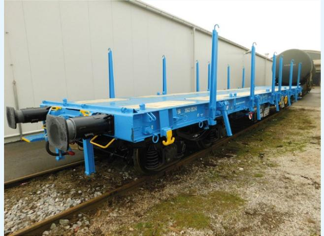
In 2016 our workshop in Dobova finished a first-time overhaul of Regmms, a type of Class R flat wagons intended for container transport and timber haulage, for the Czech client LOKO TRANS s.r.o. A total of twelve units were delivered to the shop for a G4.0 overhaul, new paintwork, and a redesign of the exterior image for the end user from Italy. The wagons were additionally equipped with sidewall panels, with the wooden floor replaced with metal boards.
