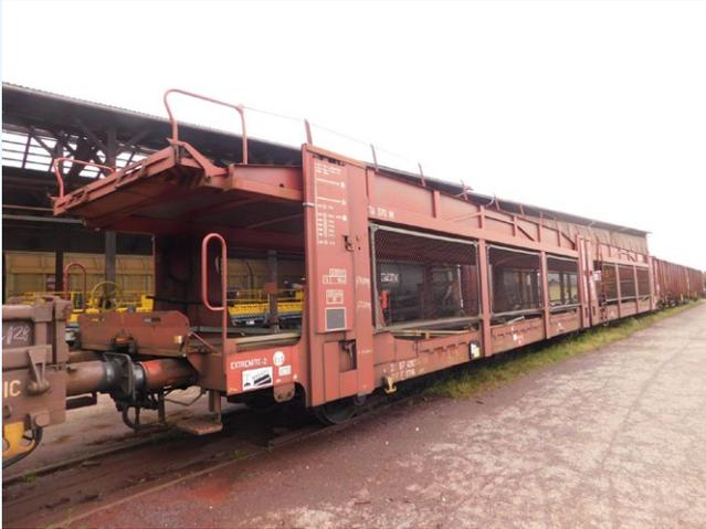
For years, the French automotive logistics company STVA has been our client in the maintenance of Laes and Laaeprs, a type of flat wagons used in car transport. Major repairs of the wagons are supplied at our shop in Dobova while routine servicing is done at Koper.
