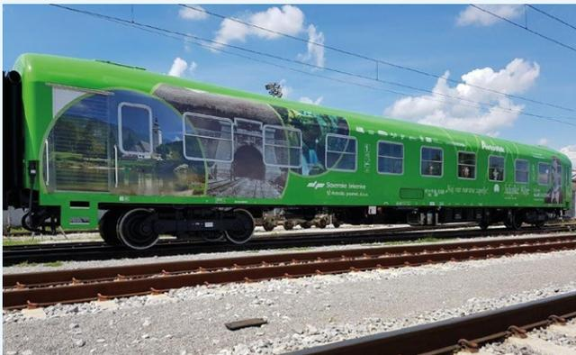
As part of an overhaul, Ptuj Center refurbished a carriage planned to run motorail service on the Soča line, a special kind of train which lets passengers take their vehicles with them on the train journey. In addition to the overhaul work, the team at Ptuj completely redesigned the carriage's interior, replacing both flooring and upholstery.
