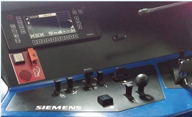
When the Global System for Mobile Communications-Railway (GSM-R) was deployed on Slovenian network at the end of 2017, the next goal was to fit the rolling stock with the associated cab radios as quickly as possible. Slovenske železnice made a decision to equip a total of 217 vehicles of 14 different types.
