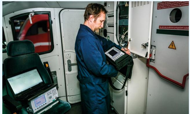
GSM-R train radio system MESA26 consists of the following components: CR26 central unit, MMIC operating device (i.e. the display), loudspeakers, handset, and the antenna. The central unit is fitted to the vehicle, with the MMIC, loudspeakers and handsets installed in the driver's cab. The antenna is fitted to the vehicle's roof. Class 643, Class 643, and Class 732 shunting locomotives are additionally fitted with gooseneck microphone and foot switch with PTT.
