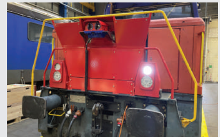
Rail Vision system mounted on locomotive
