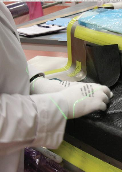
Three dimensional vision positioning system accurately projects virtual laser templates onto molds and parts to guide operators with ease through carbon fiber placement.
