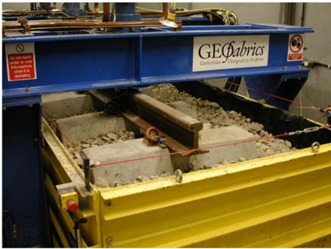
Figure 8: Large rail rig
