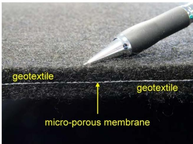
Figure 17: Geocomposite filter
