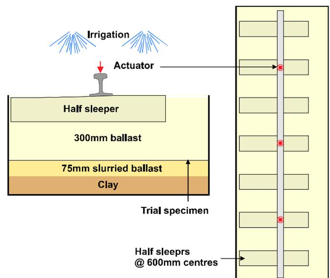
Figure 12: Test set-up on large rig
