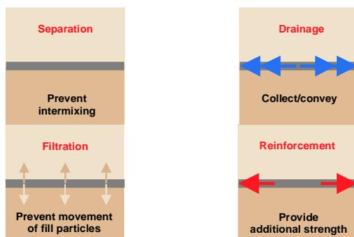
Figure 1: Principal Geosynthetic functions in rail
