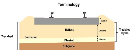
Figure 7: Current trackbed layout
