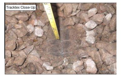
Close up of SP5 shows that where Tracktex is present, the composite is performing well and has prevented migration of the clay fines.
